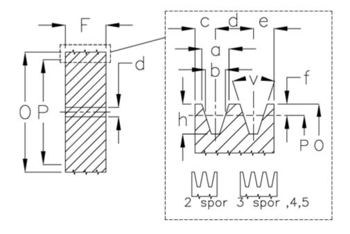
$\begin{array}{ll} d & = 15 \\ F & = 80.0 \\ Number of ribs = 5 \\ O & = 95.5 \\ P & = 90 \\ Type & = A \end{array}$
